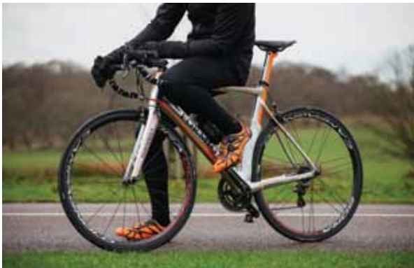
BOTTOM BRACKET The tubing on the One is sized to the maximum, making even the oversized PF86.5mm bottom bracket and chunky Super Record crank look diminutive. But it turns this to its favour – the One is stiff, yet also surprisingly comfortable.
