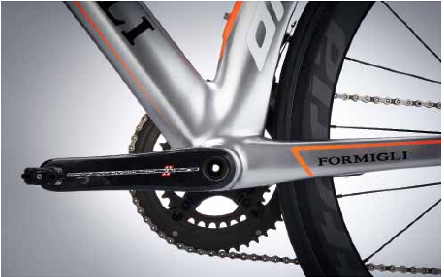
BOTTOM BRACKET The tubing on the One is sized to the maximum, making even the oversized PF86.5mm bottom bracket and chunky Super Record crank look diminutive. But it turns this to its favour – the One is stiff, yet also surprisingly comfortable.
